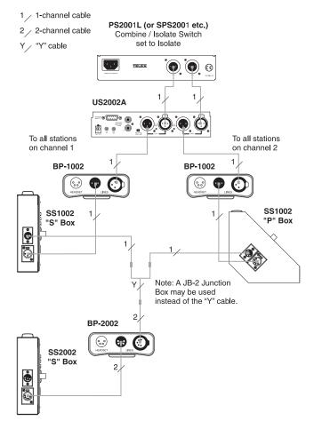
Figure 5 - An example of a phantom powered system. In this system a PS-2001L power supply is set to isolate mode. In this mode each channel is a separate party line and current per channel is limited to 1 amp. Note that both single and two channel intercom stations may be connected by using "Y" cables (or JB2 Junction boxes). Prefabricated cables may be used, or cables may be constructed using the diagrams in Figure 11.
